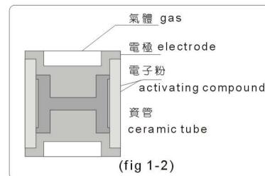
CSP series:UL-497B (Protector for data communication and fire alarm circuit)
