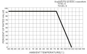
It must note one thing that the rated energy and the energy absorbed on a Varistor may not be identical. It has a situation that a ZnO varistor with better clamping voltage will absorb less energy.
